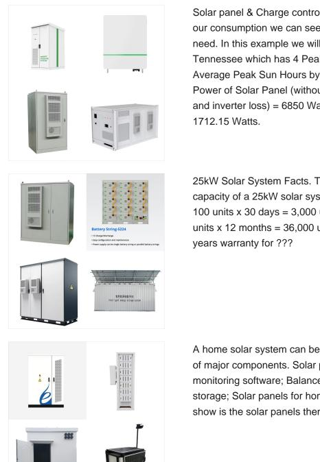
Solar panel & Charge controller. Now that we have our consumption we can see how many panels we need. In this example we will be located in Tennessee which has 4 Peak Hours (reference: Average Peak Sun Hours by State). Required Power of Solar Panel (without considering controller and inverter loss) = 6850 Watt-Hours/4 Hours =
