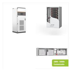
Central battery system in TKT65xxCX series, as all our Tapsa Control central battery systems, takes care of the testing automatically. Suitable for medium sized and large buildings. Technical data: input voltage 230 VAC; output voltage under normal conditions 230 VAC; output voltage in battery mode 216 VDC
