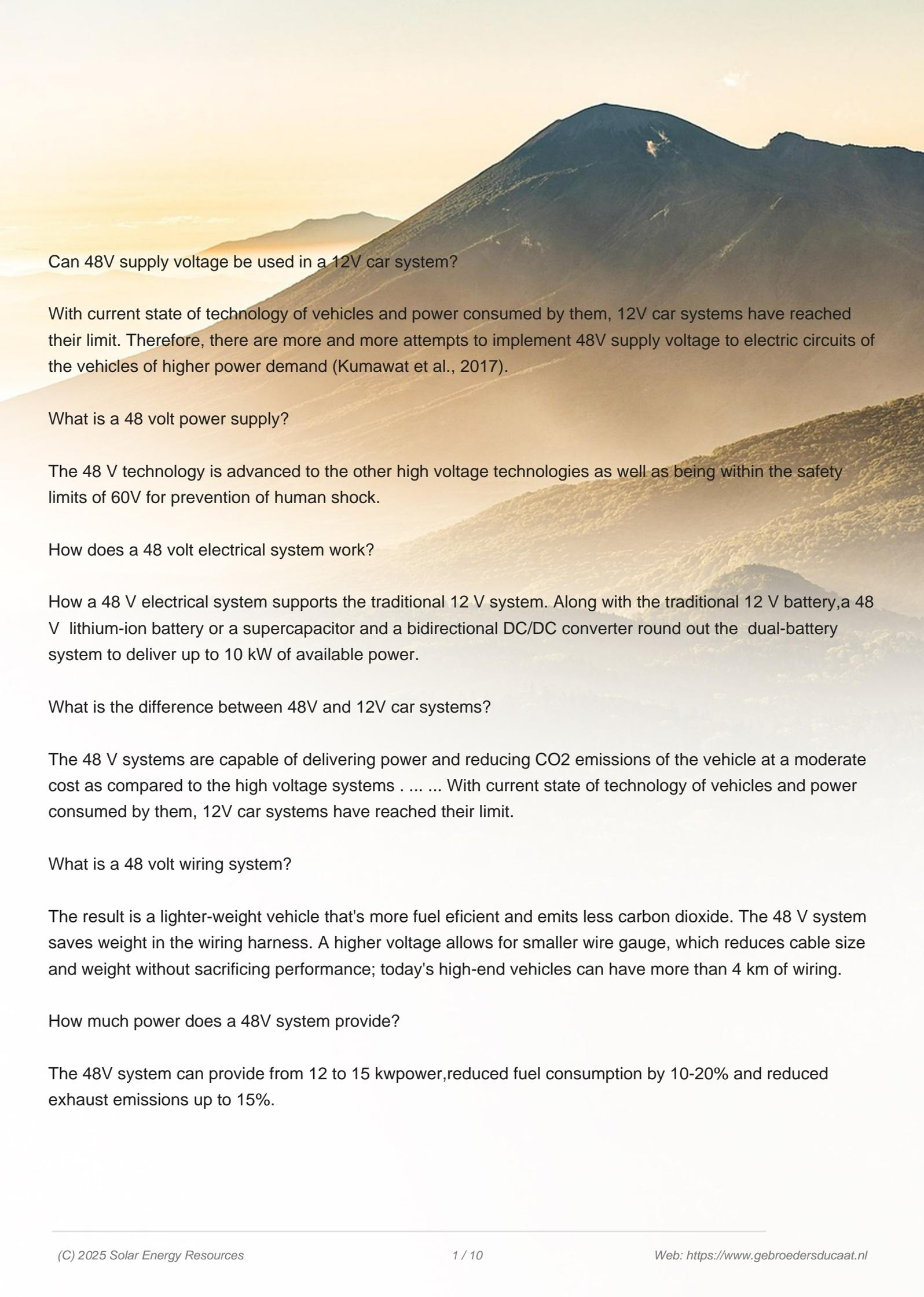
Can 48V supply voltage be used in a 12V car system?
