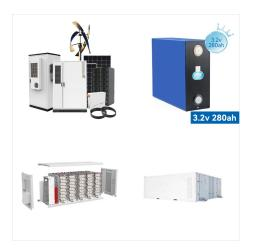
What kind of single-unit BESS are used in large-scale BESS projects? Large-scale projects use the most compact BESS containers with very high energy storage capacity. 3.727MWh in 20ft container with liquid cooling system was popular until last year which had 10P416S configuration of 280Ah, 3.2V LFP prismatic cells.
