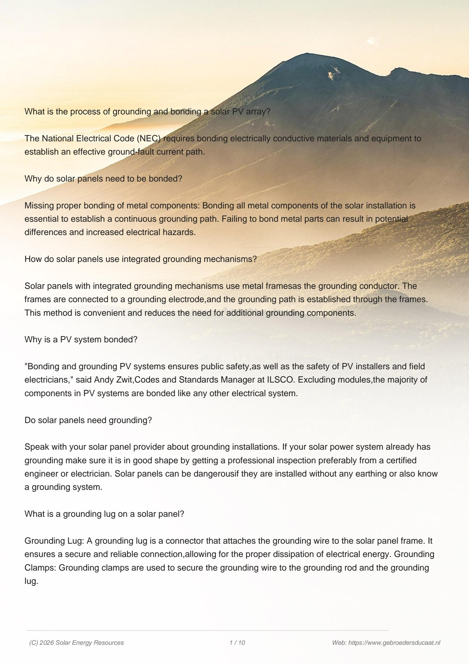
What is the process of grounding and bonding a solar PV array?
