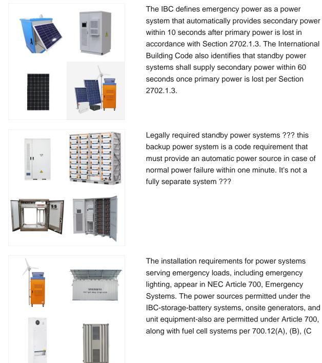
The IBC defines emergency power as a power system that automatically provides secondary power within 10 seconds after primary power is lost in accordance with Section 2702.1.3. The International Building Code also identifies that standby power systems shall supply secondary power within 60 seconds once primary power is lost per Section
