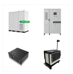
kW 1000 kWh Lithium Ion Battery Our economical, safe and long-lasting product for a wide range of applications. The E22 Li-ion battery is a containerized plug & play solution, Energy 800-1,000 kWh Maximum current (DC) 500 A 2 x 500 A Voltage range European Standard 610-820 V American Standard 670-820 V Communication interface Modbus
