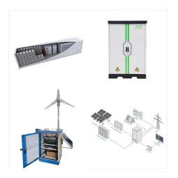
An uninterruptible power supply (UPS) and energy storage systems such as batteries are used as power backup for power interruption and disturbances. The incoming AC power has to be converted to DC for storage. When power interruption occurs, power backup converts stored DC power to AC power.
