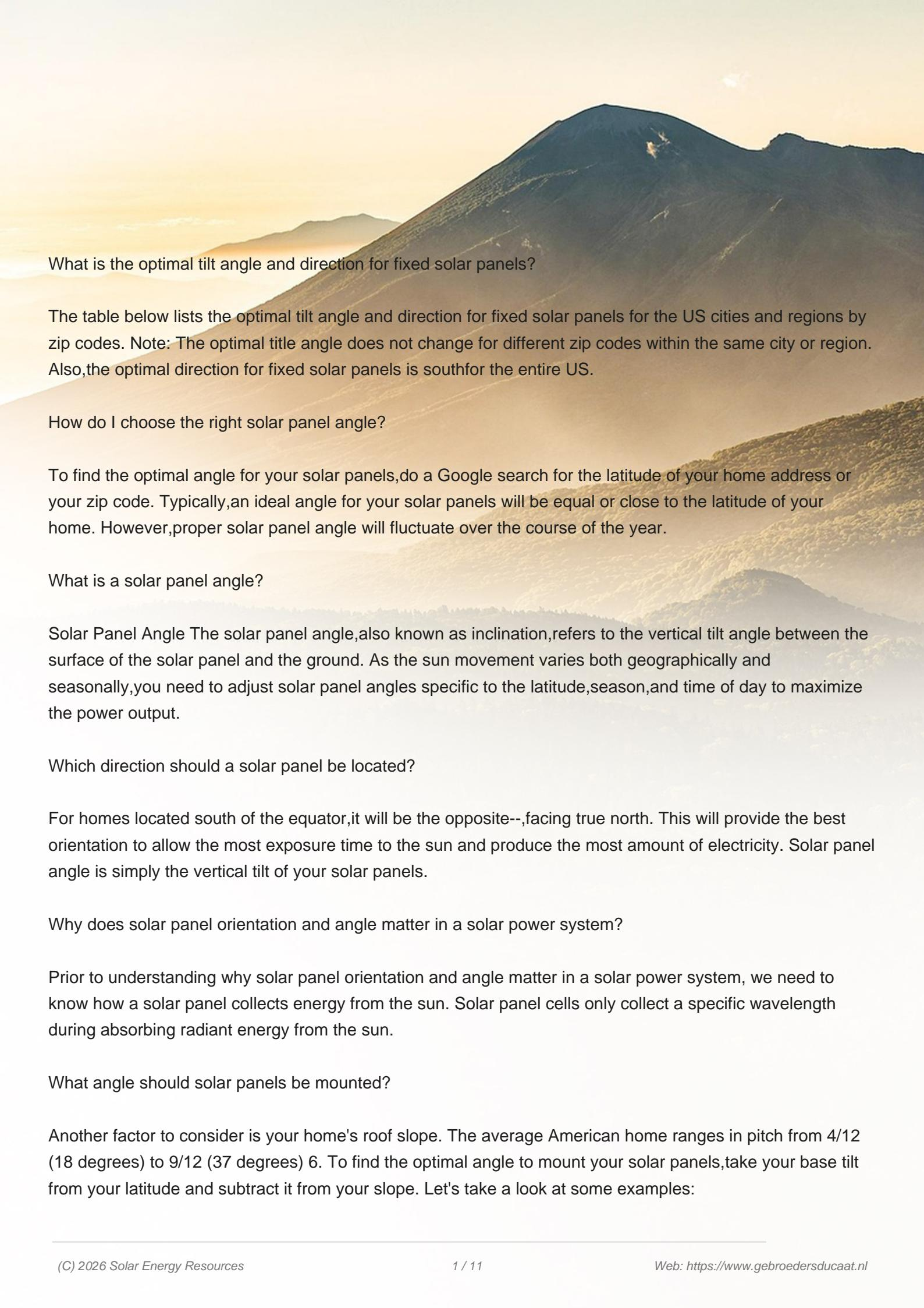
What is the optimal tilt angle and direction for fixed solar panels?
