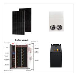
3.6 kWh Sodium-Ion battery, all integrated. 48V voltage; Only usable off-grid (isolated site) 3000 complete cycles at 100% DOD. Withstands extreme temperatures (-40? in discharge, + 65?) No risk of thermal runaway (transport to OV possible). All-in-one system with hybrid inverter, integrated solar management. 5KW continuous power
