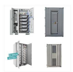
Huawei SmartLi is a Huawei-developed battery energy storage system solution that provides backup power for medium- and large-sized data centers. battery strings of different numbers of lithium batteries can be connected in parallel. Reliable. Highly stable LFP cell, no fire after thermal runaway. PACK-level fire extinguishing, precise and
