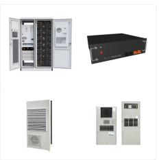
Central Battery Unit. In a centrally supplied system, the emergency and exit lights share a common power supply from a central battery unit. In its basic form, the central battery system monitors the mains voltage, maintains the charging of the batteries and supplies power to maintained luminaires in the normal mode.
