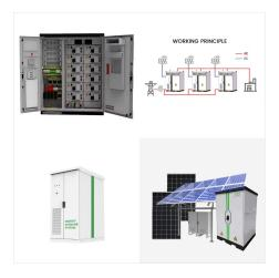
The SMA Sunny Central Storage UP battery inverter temporarily stores the surplus solar power in the battery. It performs various grid support functions including frequency, voltage and reactive power control, and it can carry out a black start in the event that the grid collapses.
