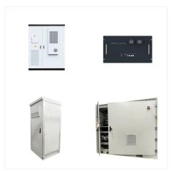
The INGECON SUN STORAGE 100TL is a three-phase transformerless battery inverter that can provide 100 kW of rated power up to 50 ?C of ambient temperature. Totally equipped The inverter is equipped with Wi-Fi and Ethernet communications as standard, as well as all the main electric protections: DC & AC surge arresters (type II), DC switch and
