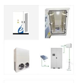
ESS-GRID series is BSLBATT's self-developed and manufactured pure battery system for commercial and industrial solar energy storage. The 100kWh battery system consists of 10 series-connected LiFePO4 51.2V 205Ah batteries controlled by a high voltage box, and it can be used in conjunction with a power conversion system (PCS) and an integrated PV storage inverter.
