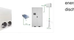
What is grid-scale battery storage? Battery storage is a technology that enables power system operators and utilities to store energy for later use. A battery energy storage system (BESS) is an electrochemical device that charges (or collects energy) from the grid or a power plant and then discharges that energy at a later time
